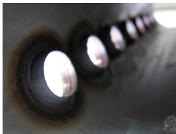
Fig. 7-4: centerdrill with pre-hole
